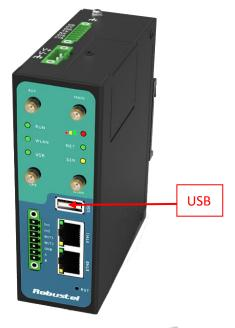
USB interface is used for batch firmware upgrade, cannot used to send or receive data from slave devices which with USB interface. Users can insert a USB storage device, such as U disk or hard disk, into the
